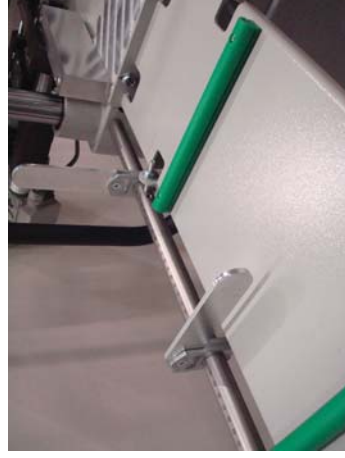
2) Lateral supports L=1/2/2,5m with 6+6 stop devices on bars with metric ruler (can't be used together with 3)
