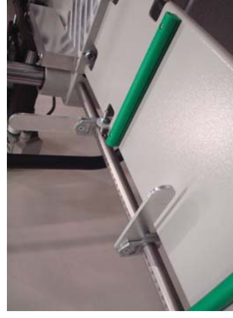
2) Vertical unit handling lever: recommended to work aluminium
