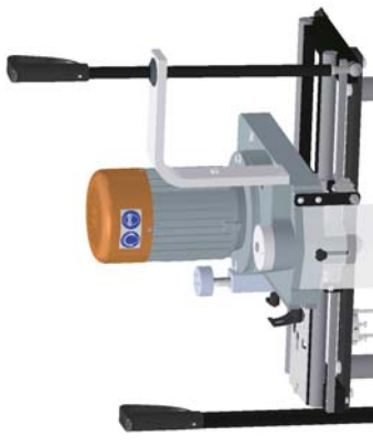
2) Vertical unit handling lever: recommended to work aluminium
