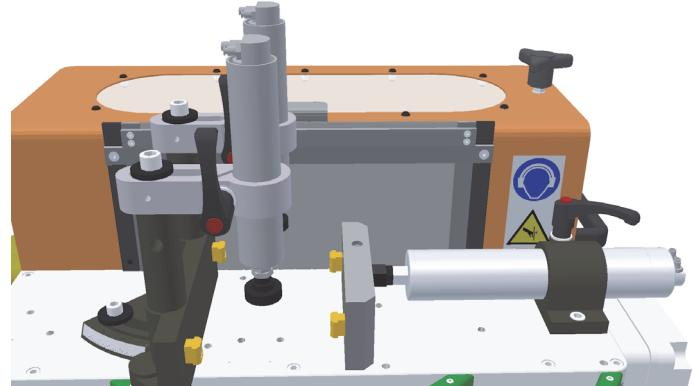
An optional horizontal clamp (code 502507) enables to block the profile at angles from 45° to 135°. This clamping includes four "T" nuts acting as a guide and vertical stop for the counter shapes, which can be inserted and replaced within few seconds.
