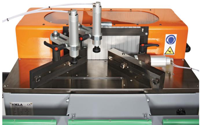
The nickel-clad, ground and polished working surface guarantees ultimate smoothness and scratch-resistance.
